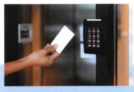
Access Control is available from a Single stand alone door to multiple doors with varied access levels. Access can be controlled via Fob or Card and the Access Card can incorporate the Staff ID.
